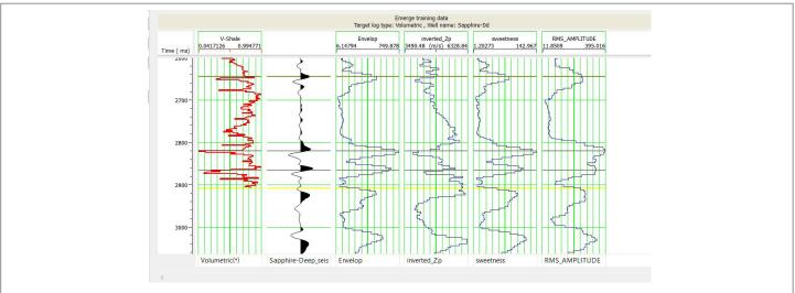
Figure 10: Analysis of target log(red) shale content, seismic trace(black) Sapphire Dd, external attribute volumes trace (blue) and analysis window (horizontal yellow lines).
