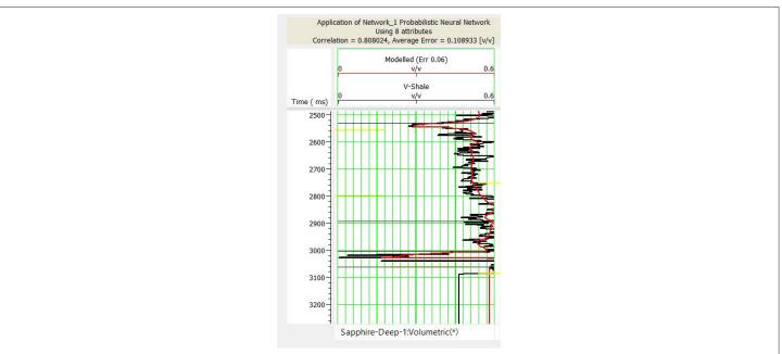
Figure 16: The application of the PNN for Vsh prediction. Measured logs are shown in black and the predicted ones are shown in red.
