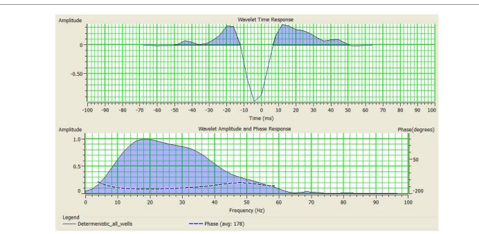
Figure 4: Deterministic wavelet using five wells used in this study with time response on top and respective amplitude spectrum on the bottom. The phase is constant 180 degree. Note: (-----) Determenistic all wells, (----) Phase (avg: 178)
