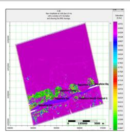
Figure 25: Relative P-Impedance slice (RMS Amplitude) on Sapphire-80. There is undrilled low water saturation (sand reservoir) that takes Sheet shape.
