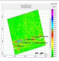
Figure 24: Relative P-Impedance slice (RMS Amplitude) on Sapphire-80. There is undrilled high effective porosity (sand reservoir) that takes Sheet shape.
