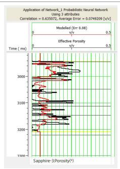
Figure 17: The application of the PNN for effective porosity prediction. Measured logs are shown in black and the predicted ones are shown in red.
