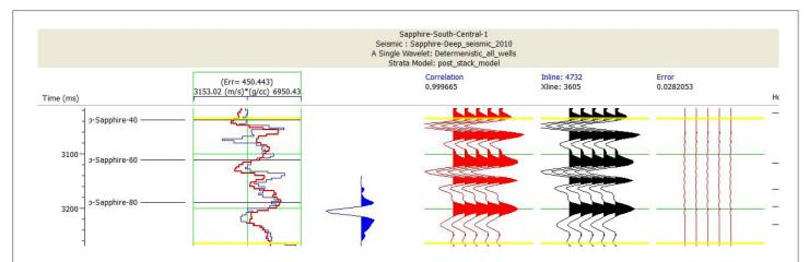
Figure 7: Post-stack inversion analysis for well Sapphire South Central using deterministic wavelet. Showing the inversion analysis was done for the reservoir interval in Sapphire 40 to Sapphire 80.
