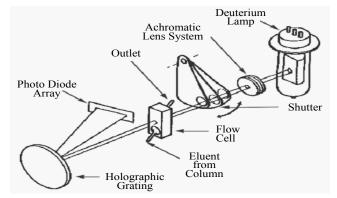
Figure 6: UV detector for liquid chromatography (would be similar for MEKC).
