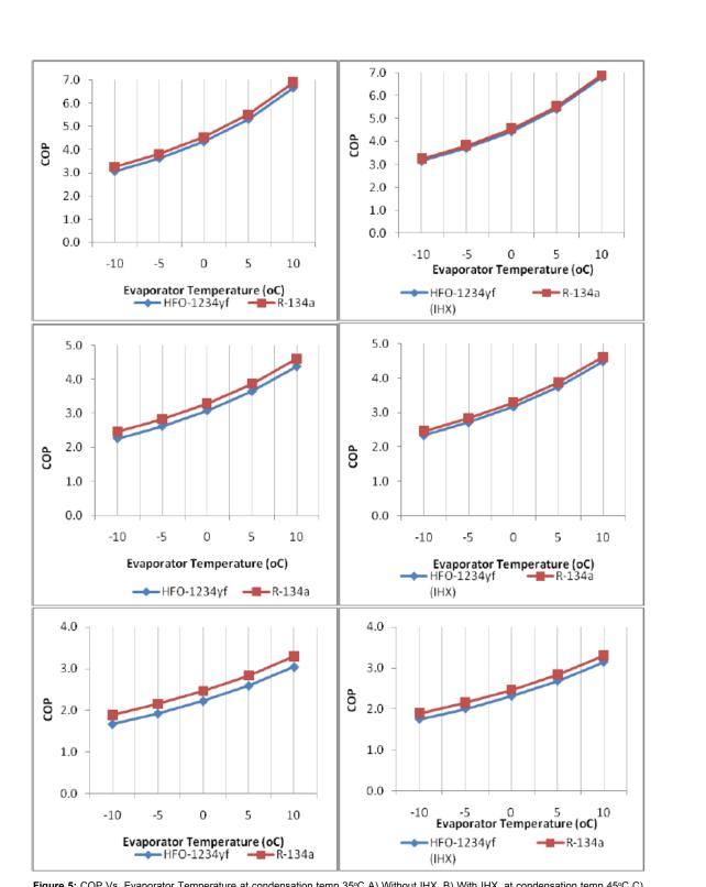
Figure 5: COP Vs. Evaporator Temperature at condensation temp  $35^{\circ}C$  A) Without IHX, B) With IHX, at condensation temp  $45^{\circ}C$  C) Without IHX & D) With IHX and at condensation temp  $55^{\circ}C$  E) Without IHX and F) With IHX.
