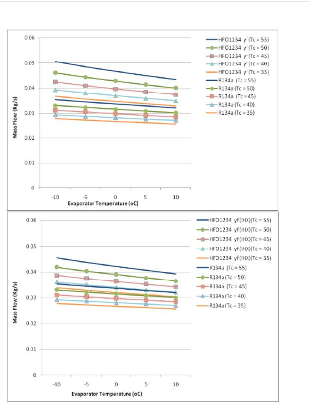
Figure 6: Theoretical Mass flow rate Vs. Evaporator Temperature (At varying condenser temp) (with and without heat exchanger).
