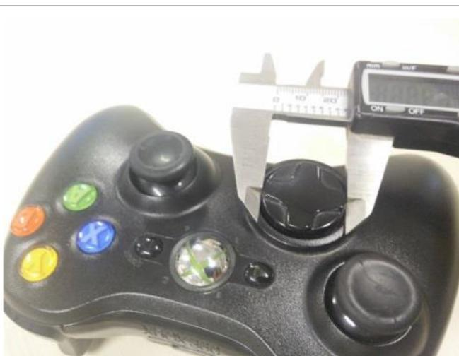
Figure 13: Diameter of the directional pad.
