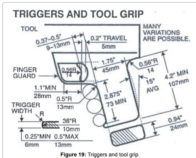
Figure 19: Triggers and tool grip.
