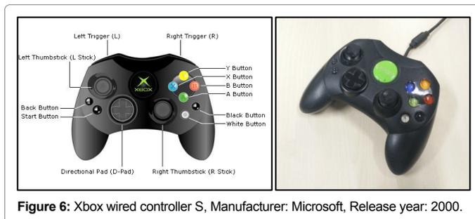
Figure 6: Xbox wired controller S, Manufacturer: Microsoft, Release year: 2000.
