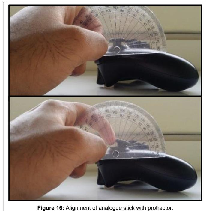
Figure 16: Alignment of analogue stick with protractor.
