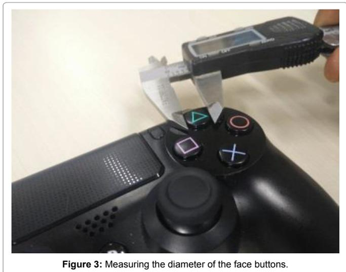
Figure 3: Measuring the diameter of the face buttons.
