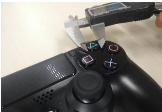
Figure 11: Buttons width/diameter measurement with Vernier calliper.
