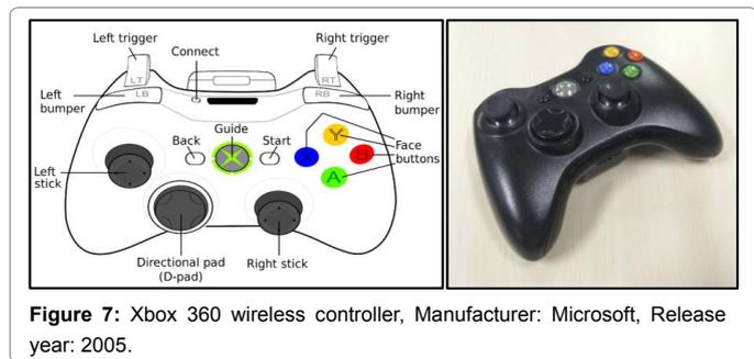
Figure 7: Xbox 360 wireless controller, Manufacturer: Microsoft, Release year: 2005.
