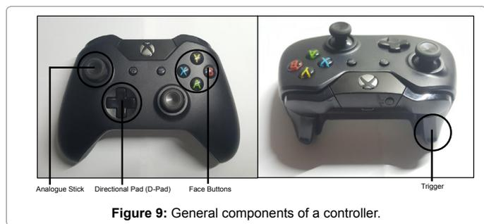
Figure 9: General components of a controller.
