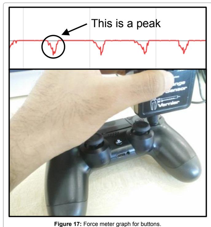
Figure 17: Force meter graph for buttons.
