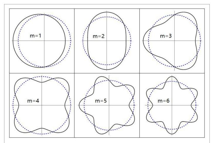
Figure 1: Possible earth's orbits (a/d=5). The dashed line represents the trace of the ideal rotor, and the solid line represents the composite trace of the rotor and vibrator.
