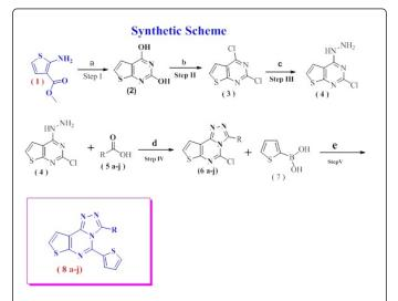
**Figure 2:** Synthetic path way for compounds 8a-8j. Synthetic path way of preparation of 1,2,4-triazole thienopyrimidine derivatives. Reagents and Reaction conditions: (a) Urea 200°C, 3 hrs (b) POCl<sub>3</sub>, N-ethyl - N, N di isopropyl amine Reflux, 6 hrs (b) Hydrazine hydrate, Tri Ethyl Amine, Ethanol, 0°C-RT, 3 hrs. (d) POCl<sub>3</sub>, Reflux, 6 hrs (e) 1,4-Di oxane, Na<sub>2</sub>CO<sub>3</sub>, Water, Pd(PPh<sub>3</sub>)4, RT-110°C, 12 hrs.
