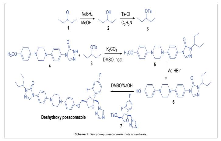
methoxy triazole compound (4) to afford the corresponding triazole alkylated derivative (5), which was demethylated by using aqueous HBr to give the phenolic compound (6). The phenolic compound (6) was reacted with tosyl derivative (7) under basic conditions to afford deshydroxy posaconzole. The obtained deshydroxy posaconazole structure was confirmed by <sup>1</sup>H NMR, <sup>13</sup>C NMR, IR and mass spectra.
