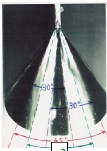
View n 3 [33-54-57] \beta = 68.6^\circ i = 45^\circ 19000 < Re < 80000
