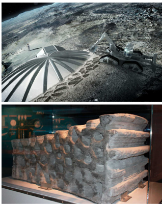
Figure 8: Proposal from Foster and Partners for a 3D-printed, lunar habitation, with a detail from the experimental, cellular structure.
