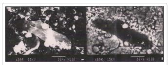
Figure 10: SEM-microphotograph of carbon soot-particle in patina layer above open-space Campanian chert breccia (0.5 km SE of Arad): (4095) SEI, (4096) backscatter.
