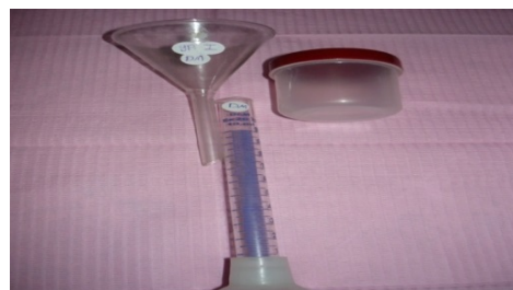
Figure 1: Tubes graduated in milliliters, a glass funnel and a plastic container used for saliva collection.
