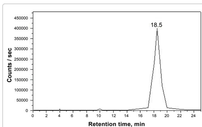
Figure 14: In-vitro stability of  $^{99m}\text{Tc}$ -tricarbonyl PA (96%) at optimum condition.
