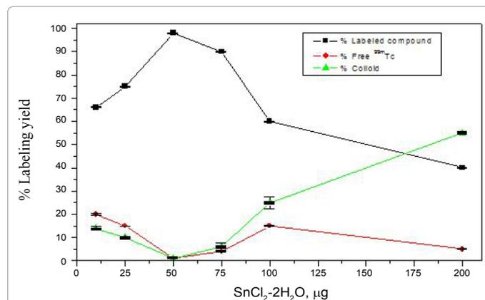
Figure 8: Effect of  $\text{SnCl}_2 \cdot 2\text{H}_2\text{O}$  amount on the radiochemical yield % of  $^{99m}\text{Tc}$ -phthalic acid.
