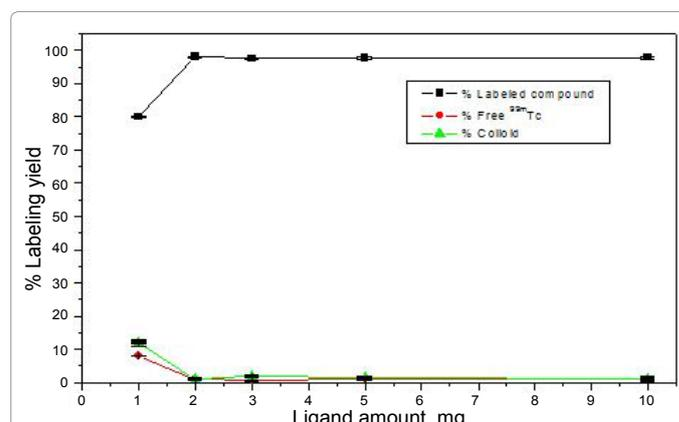
Figure 9: Percent radiochemical yield of  $^{99m}\text{Tc}$ - phthalic acid as a function of substrate amount.
