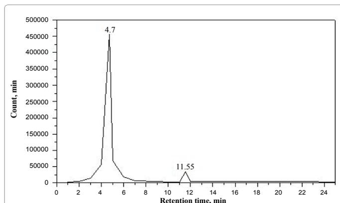
**Figure 6:** HPLC radiochromatogram of  $[\text{Tc}(\text{CO})_5(\text{H}_2\text{O})_3]^+$  precursor, pH = 11, flow rate 0.6 ml/min,  $R_t = 4.5$  min for  $[\text{Tc}(\text{CO})_3(\text{H}_2\text{O})_3]^+$ ,  $R_t = 11.44$  min for free  $^{99m}\text{TcO}_4^-$  using 0.22  $\mu\text{m}$  millipore filtration to eliminate unknown radiochemical impurities.
