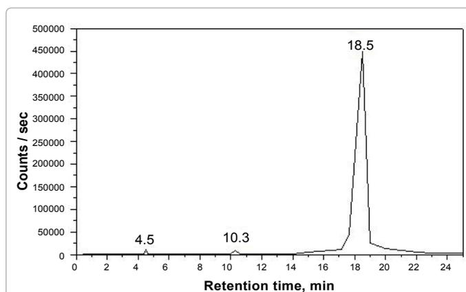
Figure 15: In-vitro stability of  $^{99m}\text{Tc}$ -tricarbonyl PA in serum at  $37^\circ\text{C}$ .
