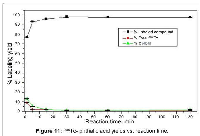
Figure 11:  $^{99m}\text{Tc}$ - phthalic acid yields vs. reaction time.
