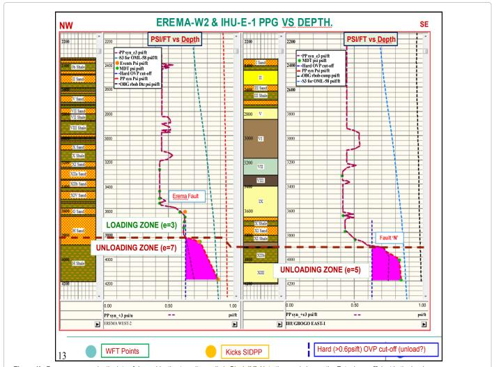
Figure 1b: Pressure versus depth plots of deep objective targeting wells in Block "X". Note the need change the Eaton's co-efficient in the hard overpressure zone.
