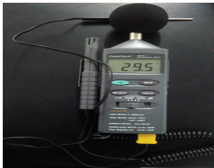
Figure 2: Environmental Monitor Meter.
