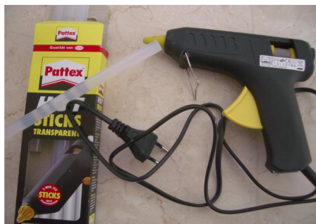
Figure 2: Pattex®-Henkel KGaA melting apparatus (Nr: 10172786 Duesseldorf, Germany).
