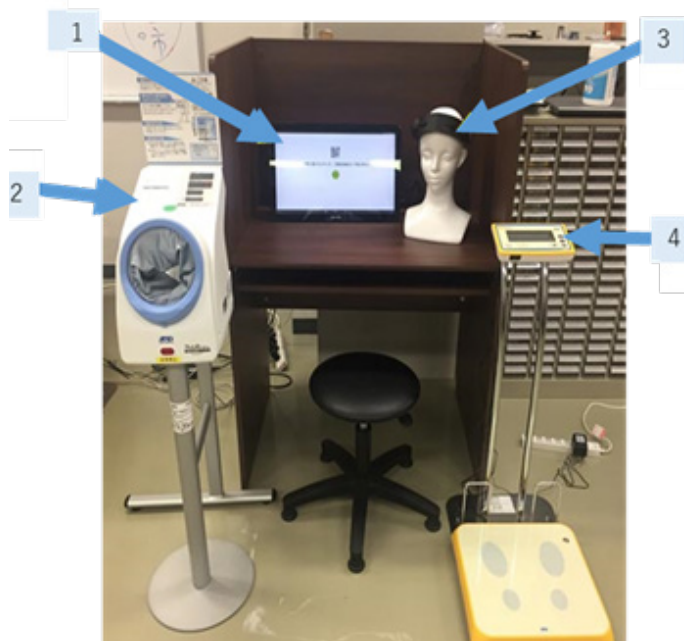
Figure 3: IoMT system. 1 Control PC, 2 Sphygmomanometer(TM-2657, A&D Corp.), 3 Two-channel-NIRS (HOT-1000, Hitachi High-Technologies Corporation), 4 Weight Scale (AD-6209PBT-C, A&D Corp.)
