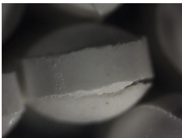
Figure 2: Delaminating on spherical mini-tablets.
