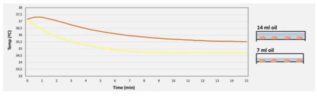
Figure 5: Oil: Temperature dynamics in a micro drop system.
