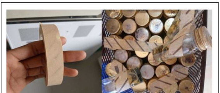
Figure 1: The autoclave tape with invisible black lines (left view) and visible black lines (right view) for quality control check of the complete media autoclaving.
