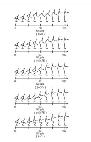
**Figure 6:** Motion patterns of lifting operation simulated with the control variable (s = 0, 0.25, 0.5, 0.75, 1).
