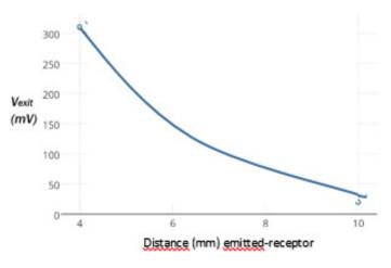
Figure 5:  $V_{\mbox{\tiny exit}}$  in function of the distance: it decreases on wider distance emitted receptor.
