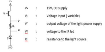
Figure 2: Diagram of the light source.
