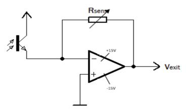
Figure 4: Electronic diagram of light sensor.
