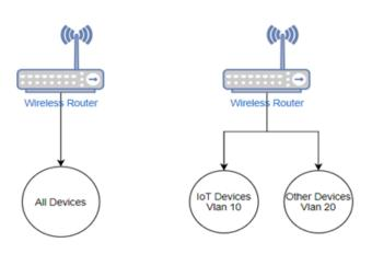
Figure 1: Non-Vlan vs Vlan.
