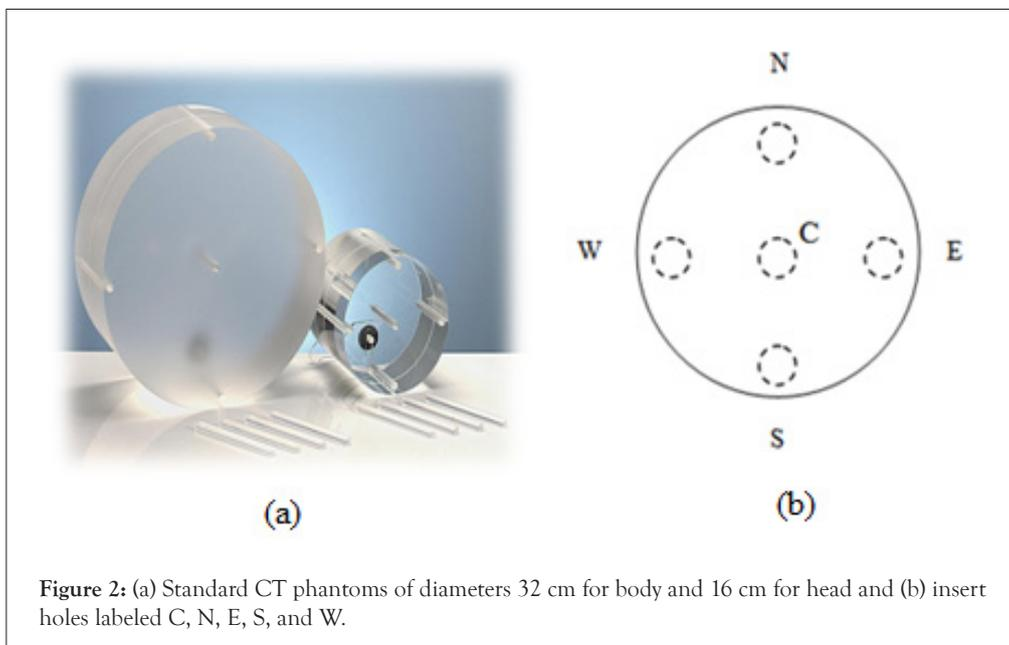
Figure 2: (a) Standard CT phantoms of diameters 32 cm for body and 16 cm for head and (b) insert holes labeled C, N, E, S, and W.
