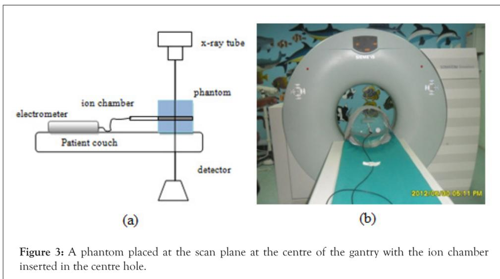
Figure 3: A phantom placed at the scan plane at the centre of the gantry with the ion chamber inserted in the centre hole.
