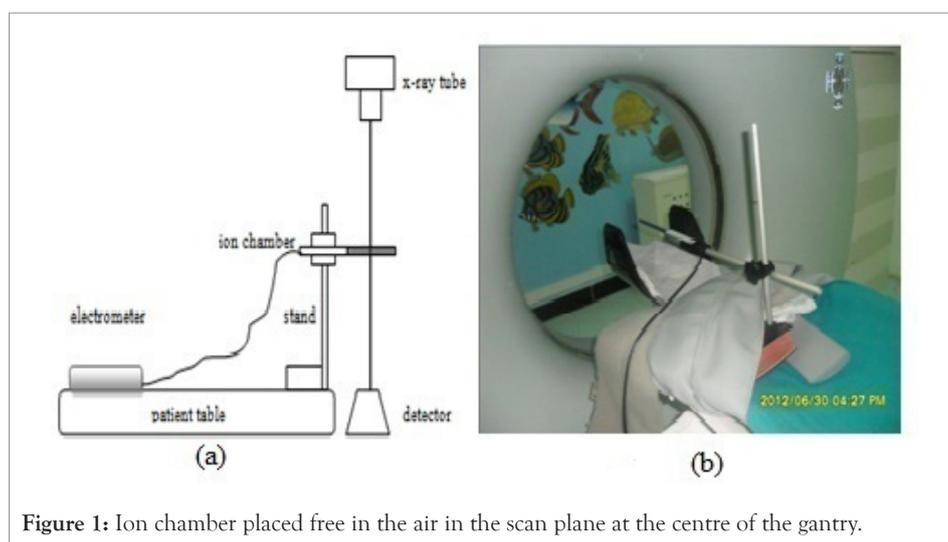
**Figure 1:** Ion chamber placed free in the air in the scan plane at the centre of the gantry.
