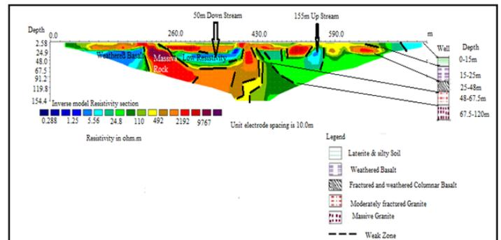
Figure 2: 2D imaging profile section of Amba-1(Hoha river above the bridge).
