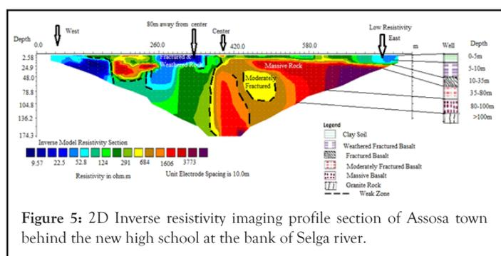
Figure 5: 2D Inverse resistivity imaging profile section of Assosa town behind the new high school at the bank of Selga river.
