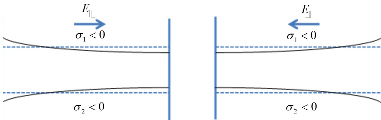
Figure 11: Membrane deformations caused by the microwave electric field parallel to the surface of the membrane; \sigma_1, \sigma_2 are the inner and outer surface charge densities.
