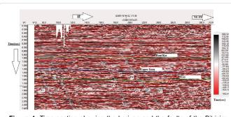
Figure 4: Time section showing the horizon and the faults of the Bitrisim area.
