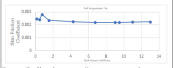
**Figure 2B:** Skin friction coefficient variation with increasing mesh resolution.
