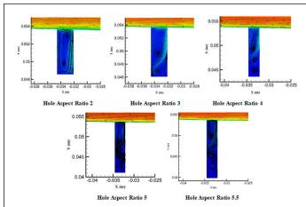
**Figure 3H:** Streamlines of the flow with variable whole aspect ratio and constant hole diameter with blowing velocity of 0 m/s around the micro-porous channel.
