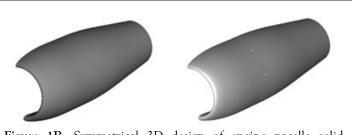
**Figure 1B:** Symmetrical 3D design of engine nacelle solid surface without micro-porous channels (left) and translucent view of micro porous-wholes (right).
