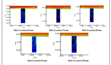
Figure 3A: Streamlines of the flow with variable whole location and constant whole diameter and aspect ratio with blowing velocity of 0 m/s around the micro-porous channel.
