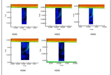
**Figure 3K:** Streamlines of the flow with variable whole diameter and constant whole aspect ratio with blowing velocity of 0 m/s around the micro-porous channel.
