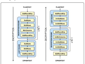
**Figure 2:** Overall structure of AES algorithm (Source: http://crypto.stackexchange.com/questions/8043/aes-addroundkey).
