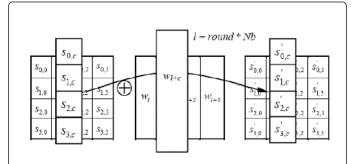
**Figure 3:** addRoundKey XORs each column of the State with a word from the key schedule.
