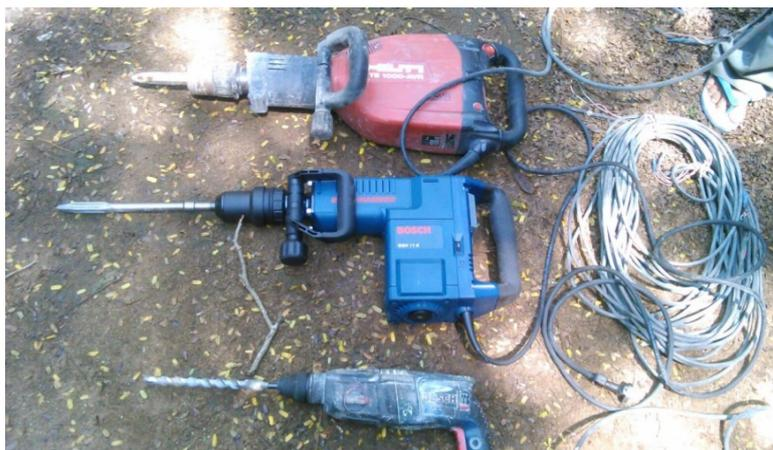
Figure 1: Types of demolition hammer used.
