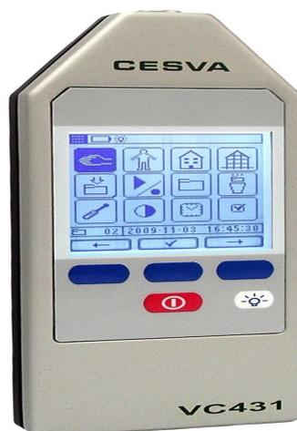
Figure 2: Vibrometercesva v431.
