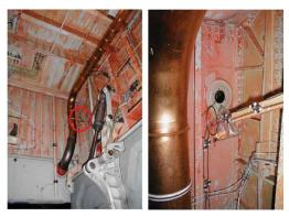
Figure 2: Center fuel tank purge door circled in red was left open by maintenance personnel [12].
