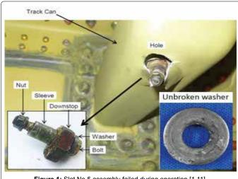
Figure 1: Slat No.5 assembly failed during operation [1,11].
