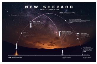
Figure 1: New Shepard flight trajectory.
