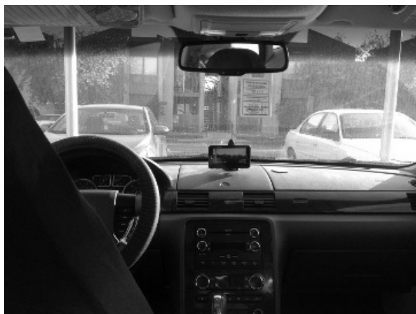
Figure 1: The system setup of the driver fatigue detection system using a smartphone.
