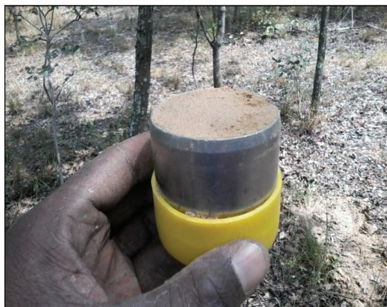
Figure 3: Soil bulk density core.
