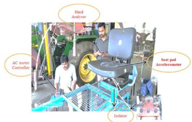
Figure 1: Setup for measuring vibration in the X, Y, Z, direction.
