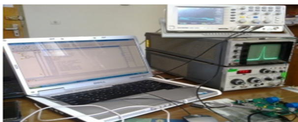
Figure 7: A depiction of the GSM mobile simulator system, operating at 940MHz.
