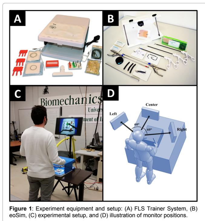
**Figure 1:** Experiment equipment and setup: (A) FLS Trainer System, (B) eoSim, (C) experimental setup, and (D) illustration of monitor positions.
