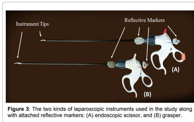
**Figure 3:** The two kinds of laparoscopic instruments used in the study along with attached reflective markers: (A) endoscopic scissor, and (B) grasper.
