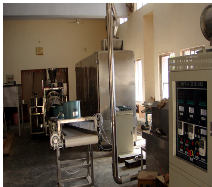
Figure 1: Pilot scale extruder units for the prepared experimental diets.
