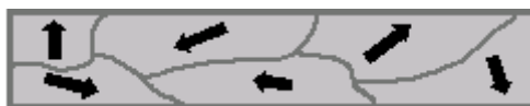
Figure 2: Magnetic domains of a magnet, when it is not attracted by any of the material. In normal case magnetic domains are like this only.
