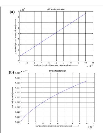
Figure 13: Variation of (a) Pore density (b) Pore radius with change in different surface tension
