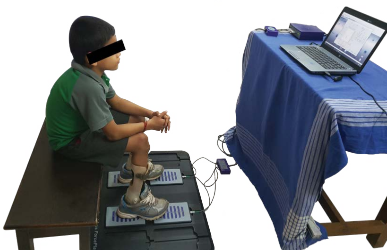
Figure 3: Starting position of the child with DAFO for the Sit to stand task on force platform.
