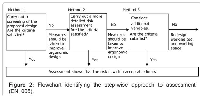
Figure 2: Flowchart identifying the step-wise approach to assessment (EN1005).
