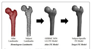
**Figure 4:** Model morphing of GHBMC M50 v4.4 femur to a subject-specific model. Homologous landmarks of the atlas (red) and subject (grey) are used to derive an interpolation function that morphs the atlas FE model to the target or subject-specific model.
