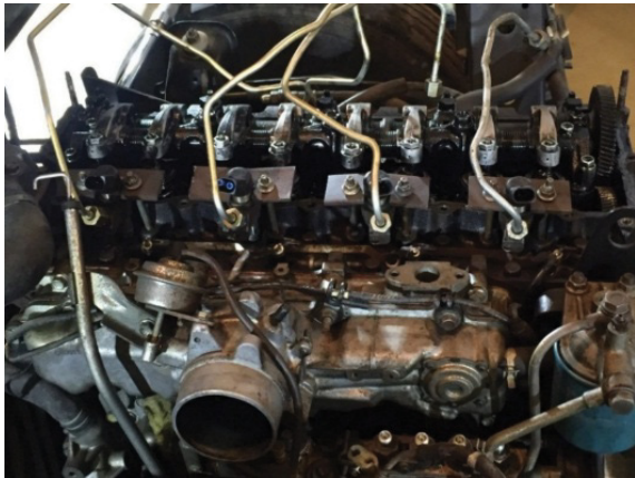
Figure 13: After installing the injectors.
