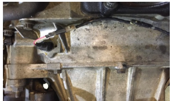
Figure 7: Testing crank sensor by oscilloscope.
