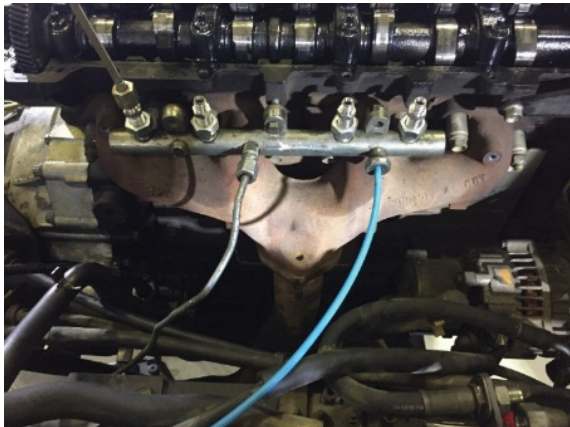
Figure 14: Installing common rail with inlet and return pipes.
