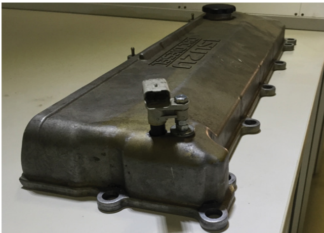
Figure 3: CAM sensor installation and testing the CAM sensor and tooth signal.
