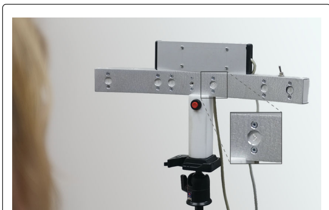
Figure 1: Reaction time perimeter showing the six visual stimulus units (large openings in the aluminum arc) constructed from 3 × 5 LED arrays assembled on a printed circuit board capable of displaying the STS (size Goldmann III) and an arrow head figure (< or >; see the inset picture) for the FO. The small opening in the centre of the aluminum arc is for an ambient light sensor for measuring the intensity of room lighting. The remote control (not in the picture) for reporting the recognition of the fixation object is connected to the perimeter by cable. Data transfer to computer was done after the test using USB cable.
