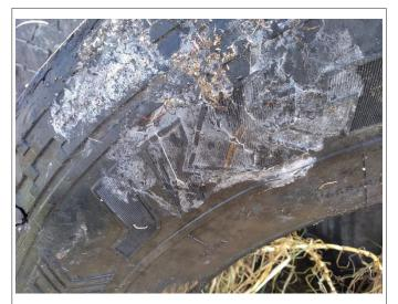
Figure 1B: Deteriorated tires with fungal growth and soil, collected on the Bogotá, D.C. Silvania, Cundinamarca route.
