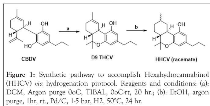
**Figure 1:** Synthetic pathway to accomplish Hexahydrocannabivarin (HHCV) *via* hydrogenation protocol. Reagents and conditions: (a): DCM, Argon purge 0oC, TIBAL, 0oC-rt, 20 hr.; (b): EtOH, argon purge, 1hr, rt., Pd/C, 1-5 bar, H<sub>2</sub>, 50°C, 24 hr.
