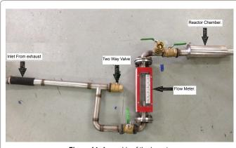
Figure 14: Assembly of the layout.
