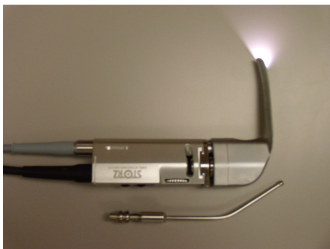
Figure 1: Video Handle containing a small TV camera incorporating the image sensor and fiber light together attached to the blade and a suction cannula with rounded tip.
