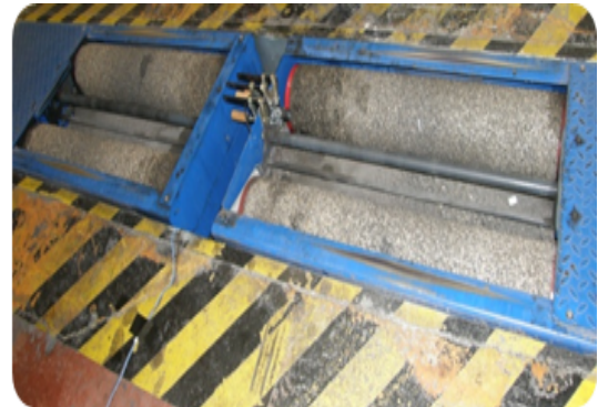
Figure 5: Roughness of rollers at MOT-450, \mu=49 \mu\text{m} .
