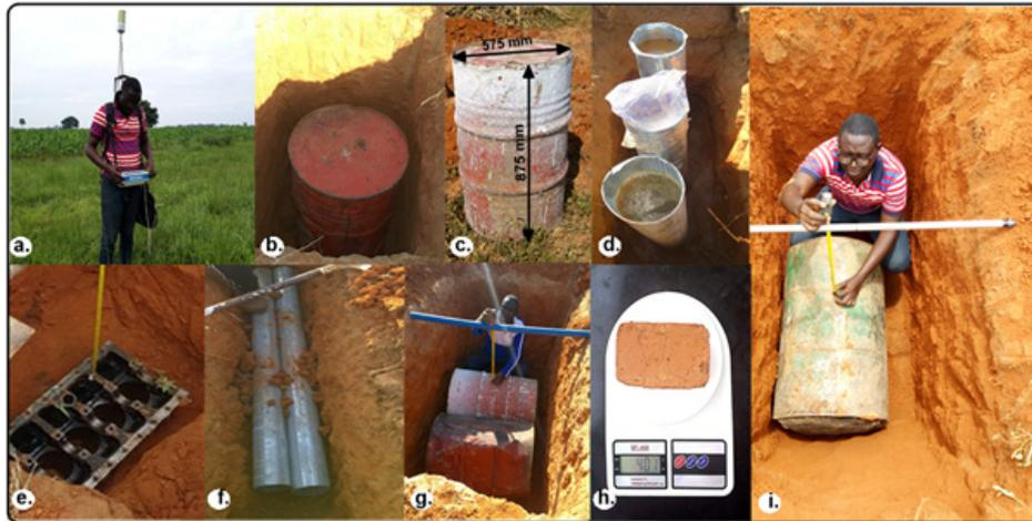
**Figure 2:** Some of the installed metallic targets and dimensions of buried targets within the GTS. (a) Magnetic surveying, (b) Vertically buried steel drum, (c) Dimensions of steel drum, (d) Three vertically buried pipes, (e) 4-cylinder engine block, (f) Two horizontally buried pipes, (g) Two horizontally buried steel drum and (h) Sample soil for density estimation, (i) Horizontally buried steel drum.
